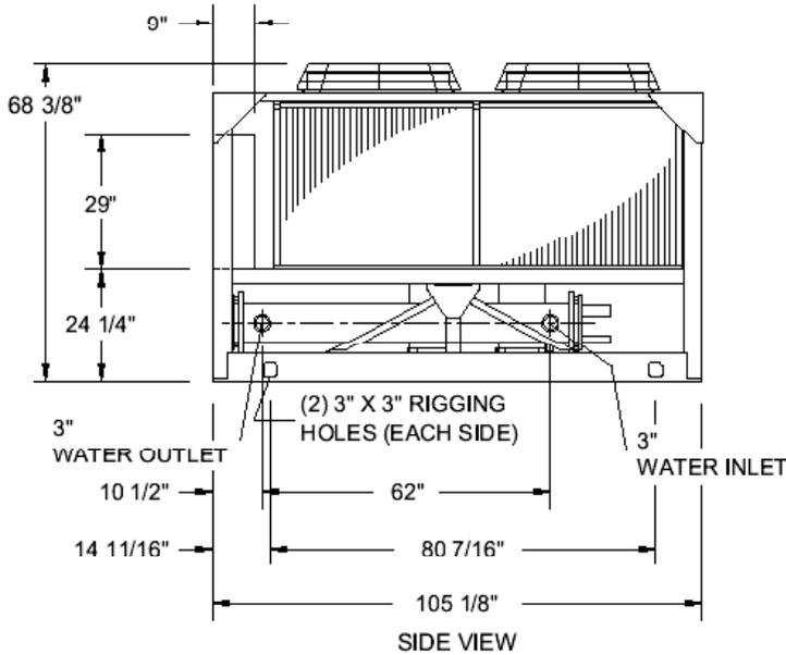
Minimum Clearances: Units Side by Side: 12 ft, Control Panel to Wall: 5 ft, Side to Wall: 8 ft, Front to Wall: 8 ft. Install unit on flat level surface.
